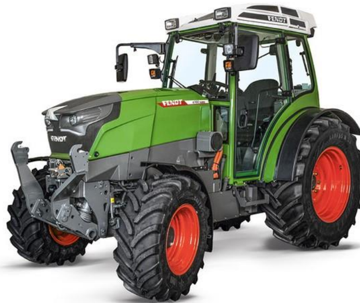
Fendt e100 Vario electric tractor (50kW / 75hp) 100 kWh battery – V2G (vehicle-to-grid) ready Field trials 2019/20 in Germany – now expected 2025
